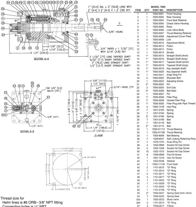
Connecting holes is 1/4" NPT Filler hole is 5/8" UNF
