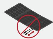
DON'T PUT ANY TENSION OR STRESS ON THE CABLES
