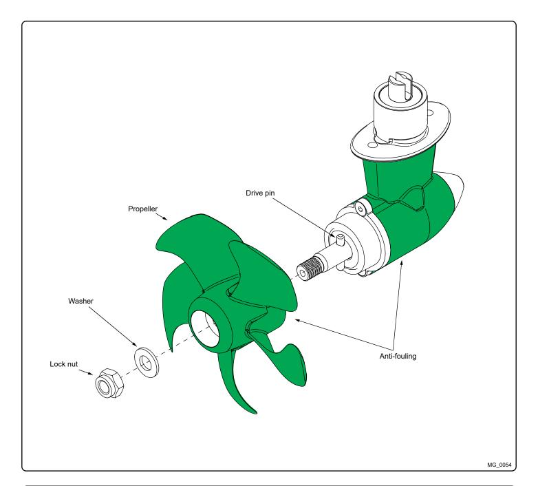
Propeller Installation MC\_0016
