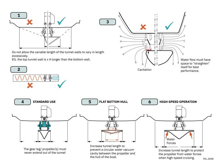
Some sail boats have a flat bottom and shallow draft in the bow section. This can make installing the thruster as far forward from the boats main pivot point difficult. (Fig. 1).
