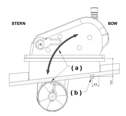
c) Once completely satisfied with the position and height of the mounting base, the base can be permanently stratified and fixed into the hull while respecting the inside dimensions of the mounting base. In order to ensure that the mounting base keeps its initial form during the stratification process, one can use some wooden spacers (length = 249 mm) on the inside of the mounting base.
