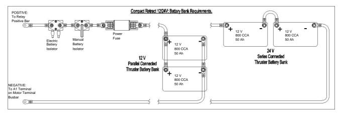
When choosing the type of batteries needed for your thruster's battery bank, keep in mind that it is the CCA (Cold Cranking Amps) capacity that is the most important and not the Ah (Amp-hour) capacity. This is because thrusters draw high currents, but only for very short periods of time (maximum 3 min.)
