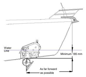
Always check and make sure that there is enough room to allow for the complete removal of the thruster unit and enough room for the connection of the electric cables.
