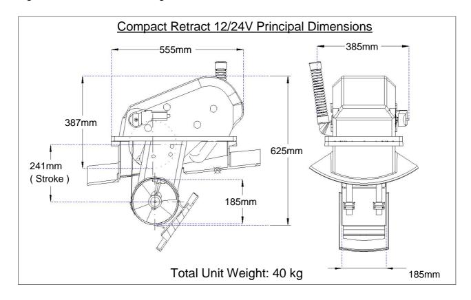
When fixing the mounting base, do not forget to take into account the overall dimensions of the Compact Retract
