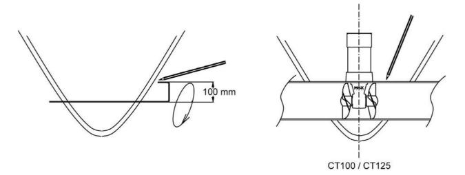
Replace the tunnel. To secure its position apply reinforced fiberglass filler to all areas, both inside and out, taking care to entirely fill the space between the hull and the tunnel. Laminate using a minimum of 8 layers of **ISOPHTALIC RESIN** alternated with mat and roving.
