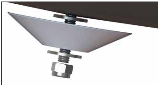
3 Use Sikaflex to seal the bolt M8
