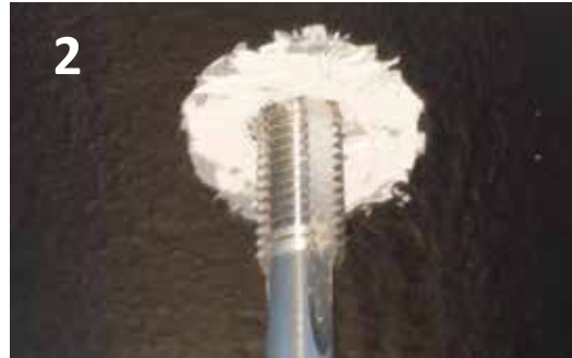
2 Drill and cut thread M8
