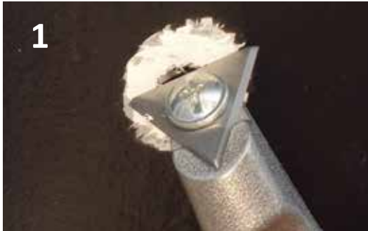
1 Remove the antifouling
