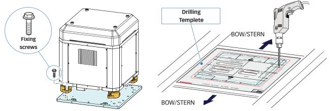
Use the drilling template supplied to mark the anchoring points before positioning the gyroscope.
