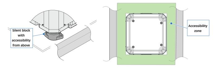
Use the drilling template supplied to mark the anchoring points before positioning the gyroscope.
