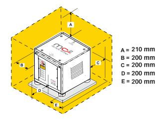
Upon request, 2D and 3D dimensional drawings can be provided to accurately assess the dimensions
