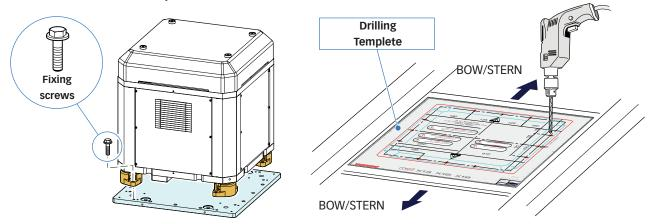
Use the drilling template supplied to mark the anchoring points before positioning the gyroscope.
