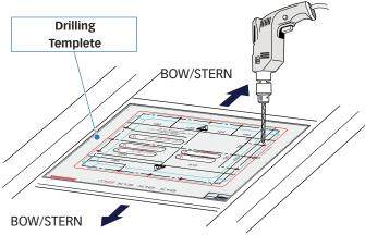
Use the drilling template supplied to mark the anchoring points before positioning the gyroscope.
