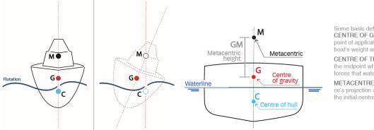
Some basic definitions: CENTRE OF GRAVITY point of application of the resultant torque of all the boat's weight and cargo.
