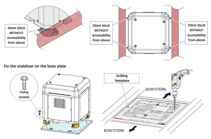
Use the drilling template supplied to mark the anchoring points before positioning the gyroscope.
