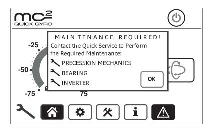
The wrench icon remains visible until maintenance is performed; despite the maintenance notice, the stabilizer will • continue to operate.
