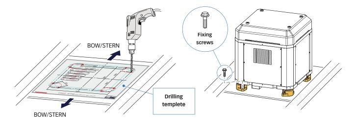
• Quick<sup>®</sup> MC<sup>2</sup>X2 shall be secured by means of screws with strength class no less than 10.9 (Grade 8), Tightening torque 136 Nm (1203.7 lbf/inch) - M12 (the screws are supplied with the product).
