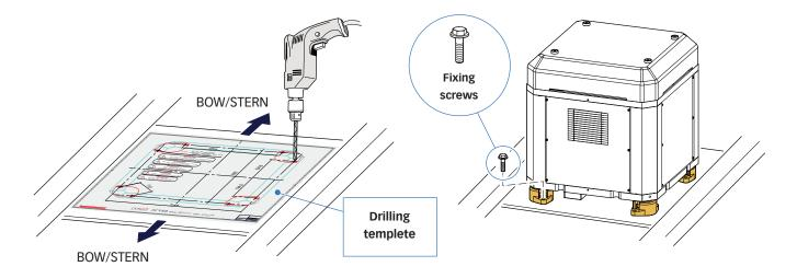
• Quick<sup>®</sup> MC<sup>2</sup>X5 shall be secured by means of screws with strength class no less than 10.9, Tightening torque 130 Nm - M12 (the screws are supplied with the product).
