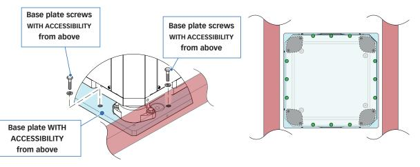
Quick<sup>®</sup> MC<sup>2</sup>X5 shall be secured by means of screws with strength class no less than 10.9, Tightening torque 40 Nm (345.179 lbf/inch) - M8\*45 (the screws are supplied with the product).
