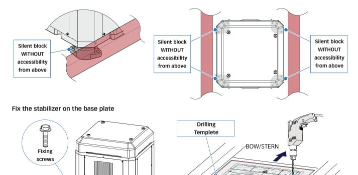
Use the drilling template supplied to mark the anchoring points before positioning the gyroscope.
