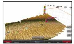
Scrolls through sonar data as the boat moves to show the history of the entire water column from the bottom to the surface and all of the fish in between.
