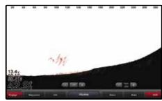
To help give you time to avoid collisions with submerged obstacles, FrontVü shows underwater obstructions within a 300' range as you approach
