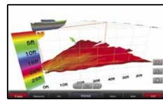
Scans the area in front of your boat, creating a forwardlooking 3-D view of the bottom, structure and fish.
